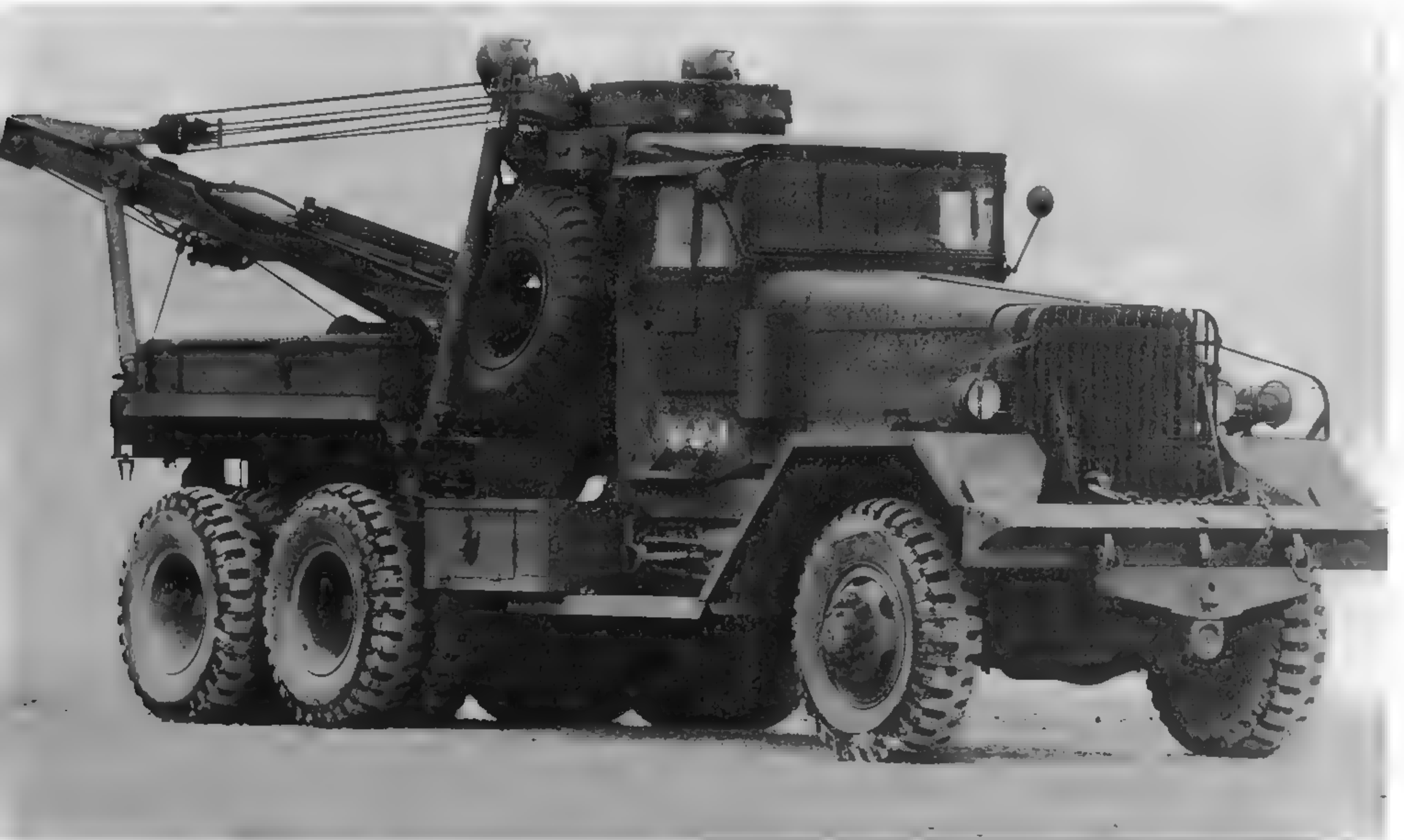
This is the Kenworth version of the M1A1. It is almost indistinguishable from a Ward LaFrance M1A1. The whiffletree was slightly different (notice the KW whiffletree lacks the flange across the back present on the Ward LaFrance). The tool lockers varied with manufacturer as well, although a few Ward LaFrances were built with the Kenworth tool lockers to use up excess inventory after Kenworth stopped building the trucks. (U.S. Army photo)
